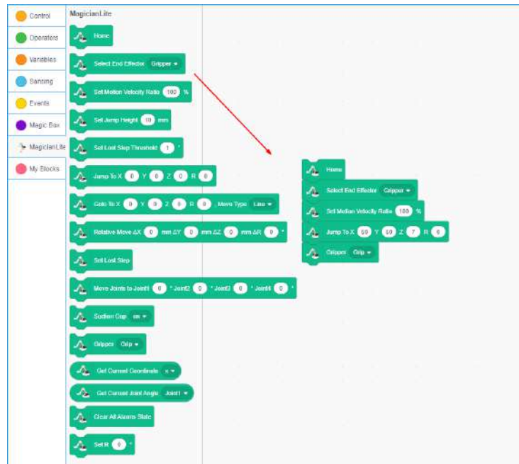
Figure 3.4 Drag blocks to the block area
